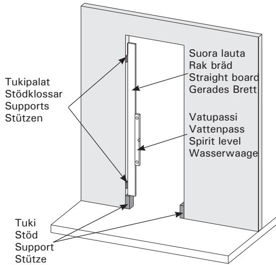
leave room for wedging on both sides of the opening. Install the supports vertically in-line using a spirit level. A straight board can be used as an extension for a short spirit level. Cut and install supports made of e.g. pieces of wood under the door.
